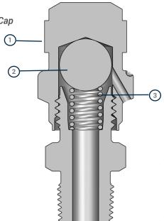
Warning! Operator should take appropriate precautions to protect themselve from system fluids that will escape during operation. The direction of the vent changes as the cap rotates. Operators should open valves slowly and ensure that system fluilds are directed away from personnel.
